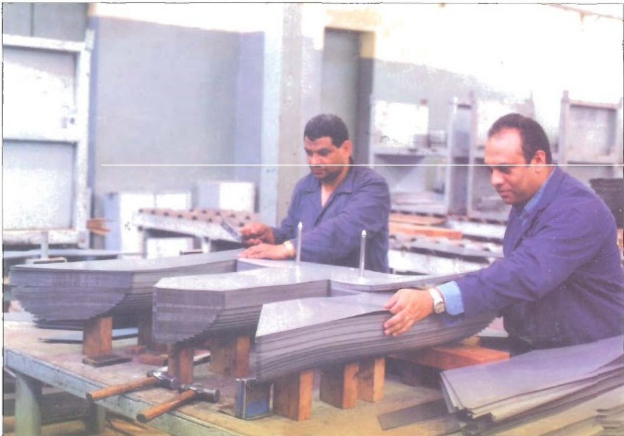
Stacking Process of Iron core
