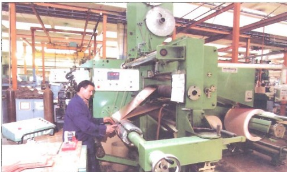
Low Voltage Winding (Foil Conductor)
